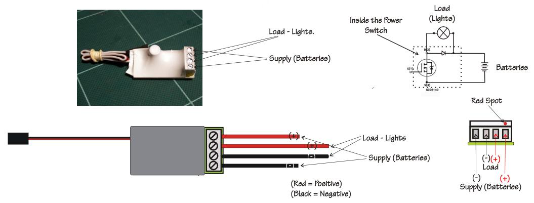
If you are using LED's you MUST fit resistors into the circuit
